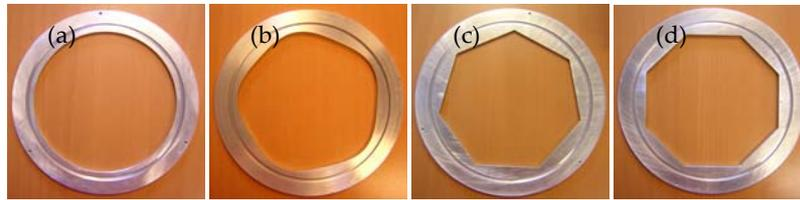
**Figure 2.** The four reflector boundaries used in the experiments, (a) a circle, (b) a smooth pentagon, (c) a heptagon and (d) an octagon.
