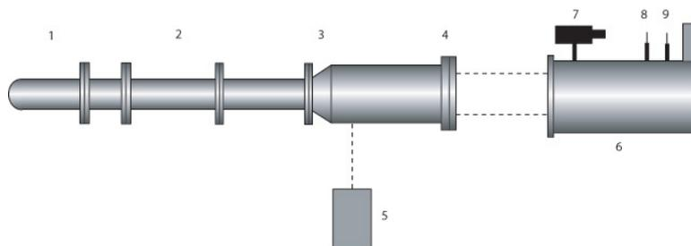
**Figure 1.** Schematic overview of the experimental setup: 1. The high pressure part, 2. Low pressure part: inlet section, 3. Low pressure part: transformation section, 4. Low pressure part: test section, 5. Pulse laser, 6. Schlieren optics, 7. PCO CCD camera, 8. Lens, 9. Schlieren edge.
