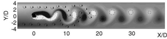
**Figure 4:** Grid UG,  $Re = 90$ , Poiseuille incoming flow, symmetry conditions imposed on the confining walls: non-dimensional vorticity, ranging from  $-0.5$  (dark grey) to  $+0.5$  (white).
