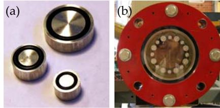
**Figure 3.** (a) the obstacles used to create disturbances in the flow field, (b) an example with  $2 \times 8$  cylinders placed in the test section.
