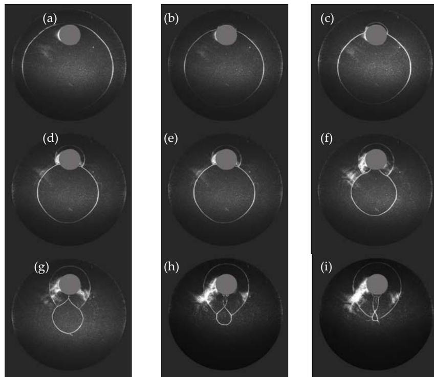
**Figure 5.** Schlieren photographs of a cylindrical converging shock wave disturbed by one cylindrical obstacle. Each photograph is from an individual run in the shock tube.
