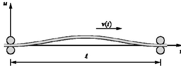
**Figure 1:** Axially moving string
