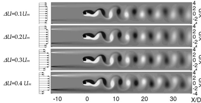
**Figure 5:** Grid UG, piece-wise constant inflow profile (sketched on the left-hand side of the figures), symmetry boundary conditions on the confining walls,  $Re_m = 90$ : instantaneous vorticity (light and dark colours stand for positive and negative vorticity, respectively).
