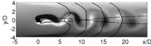
**Figure 3:** Grid SG8,  $Re = 90$ : trajectories of the wake vortices (identified as proposed in [4]).
