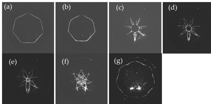
**Figure 4.** Schlieren photographs of a converging and diverging shock wave with a heptagonal reflector boundary.
