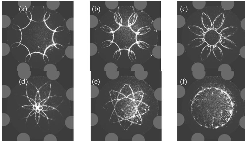
**Figure 6.** Schlieren photographs of a cylindrical converging and diverging shock wave disturbed by eight cylindrical obstacles.
