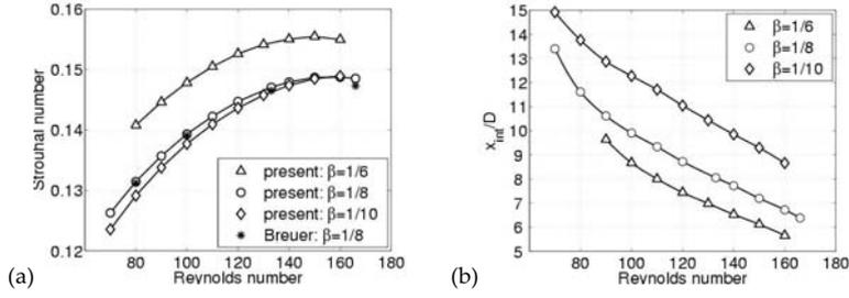
**Figure 2:** (a)  $St$  vs.  $Re$  obtained on grid SG8 and results from [1]; (b)  $x_{inv}/D$  vs.  $Re$ .
