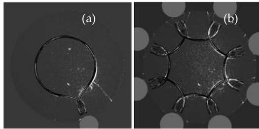
**Figure 7.** Density gradient profiles from the numerical simulations compared to experimental schlieren photographs for the case of (a) one and (b) eight cylindrical disturbances.
