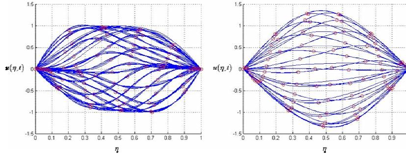
**Figure 4:** Displacements for an exponentially decaying speed: Miranker's model (left) and corrected model (right)
